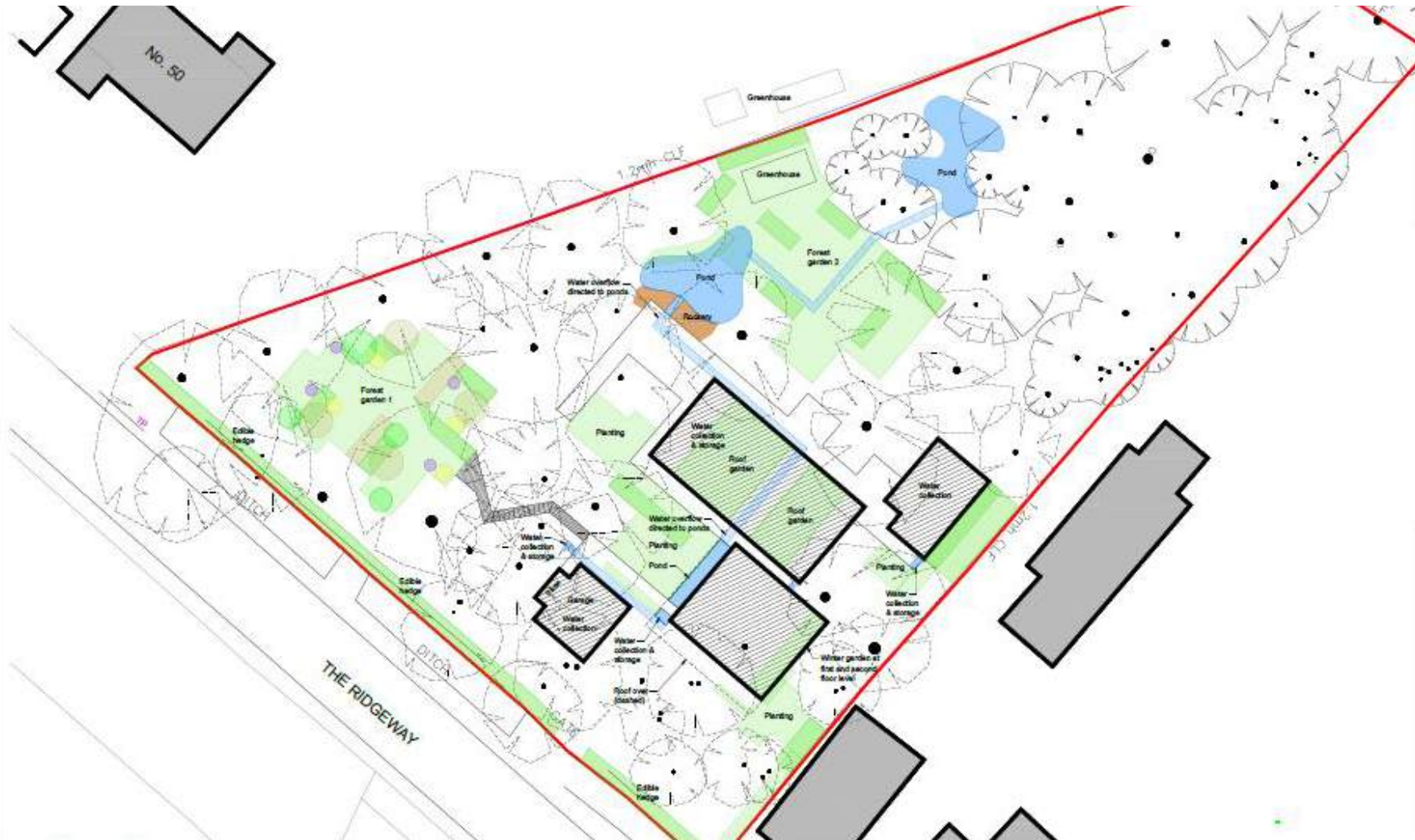
Figure 3 – Red outline boundary of the site, showing proposed ponds, forest gardens and green roof areas upon the proposed dwelling.
