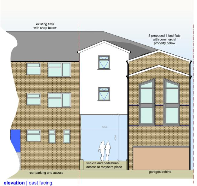
caveat: roof heights are based on brick counts and should be treated as approximate the proposal follows the existing roof ridge line terminating at the dormers.
