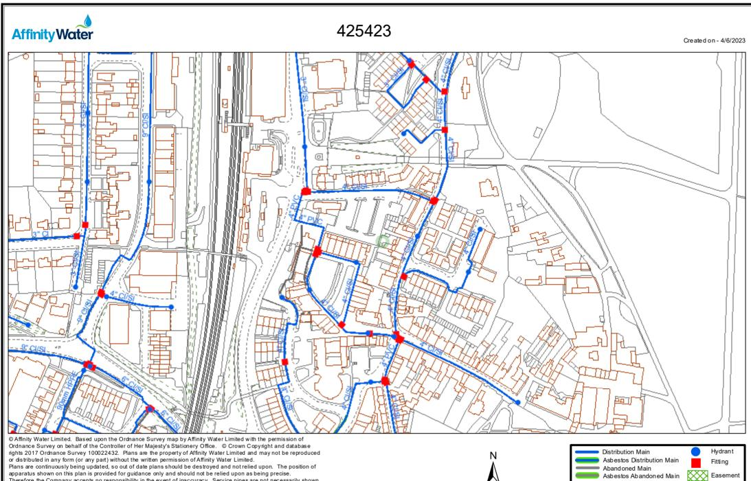
Therefore the Company accepts no responsibility in the event of inaccuracy. Service pipes are not necessarily shown on this plan. Cover is normally 915mm for mains and 750mm for communication pipes but this may vary. The actual position of apparatus must be determined on site by making hand dug trial holes. The Company requires a
