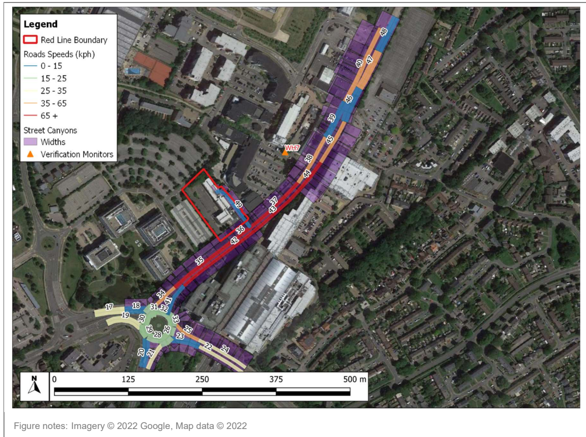
Figure 5: Modelled Road Geometries, Widths, Street Canyons and Speeds near the Proposed Development
