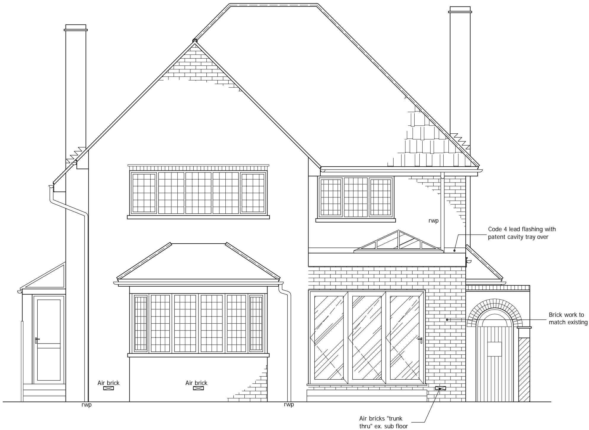
PROPOSED REAR ELEVATION scale 1:50
