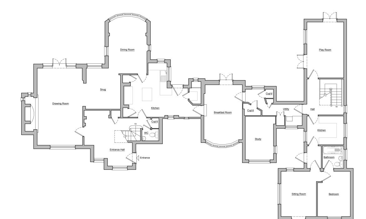
Ground Floor Plan As Existing - Scale 1:100
