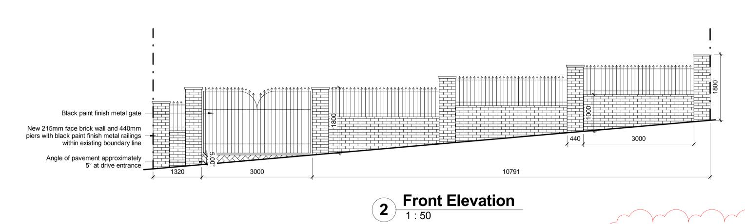
215mm face brick wall and 440mm piers with black paint finish metal railings
