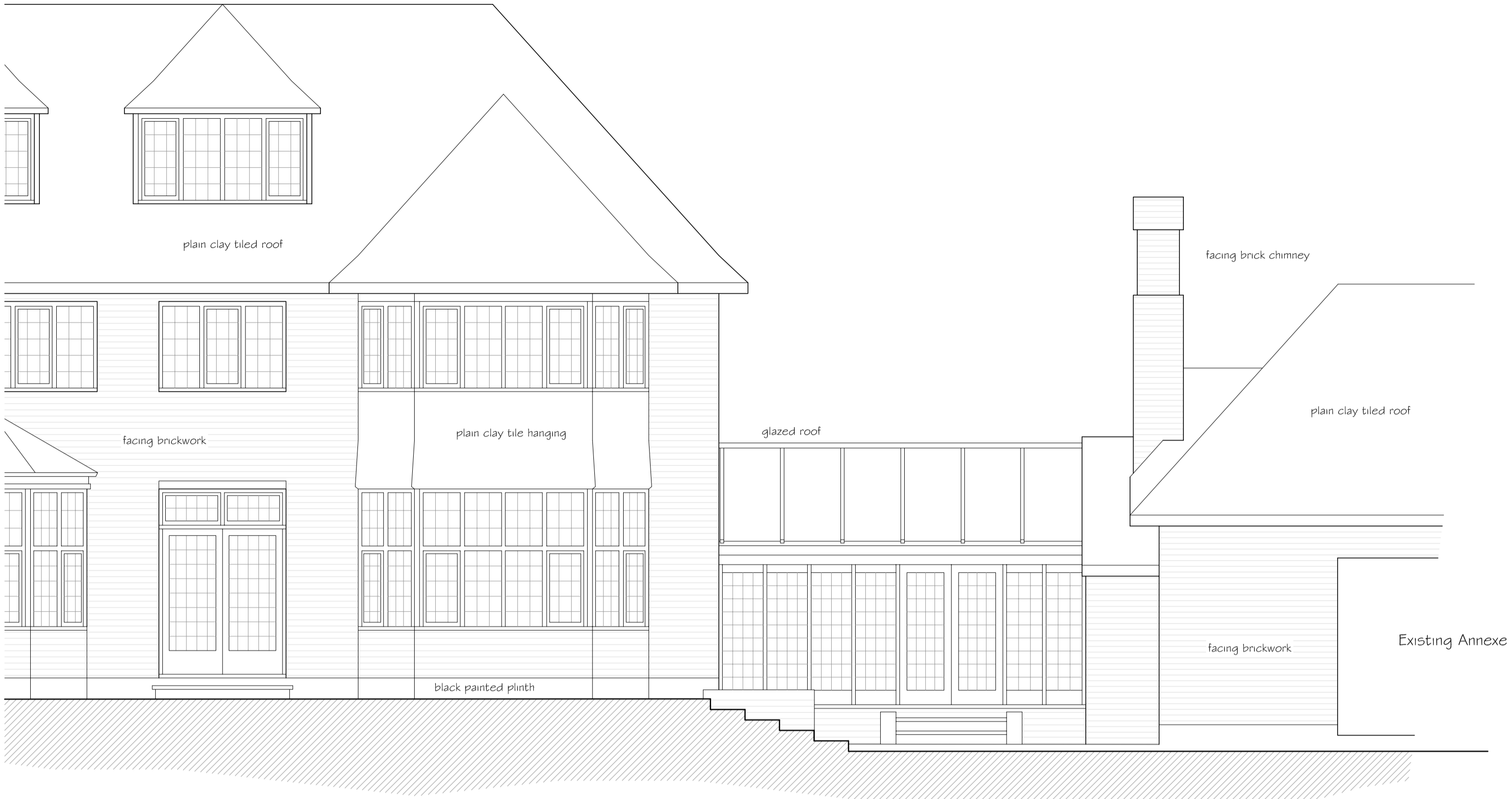
SOUTH WEST ELEVATION
