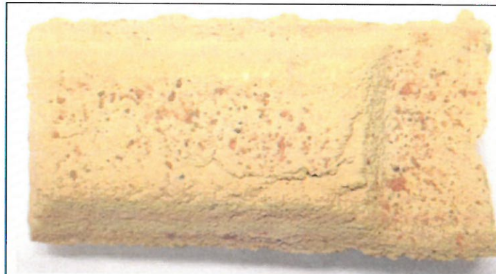
58467/1 "as received" sample showing brick contact surfaces
