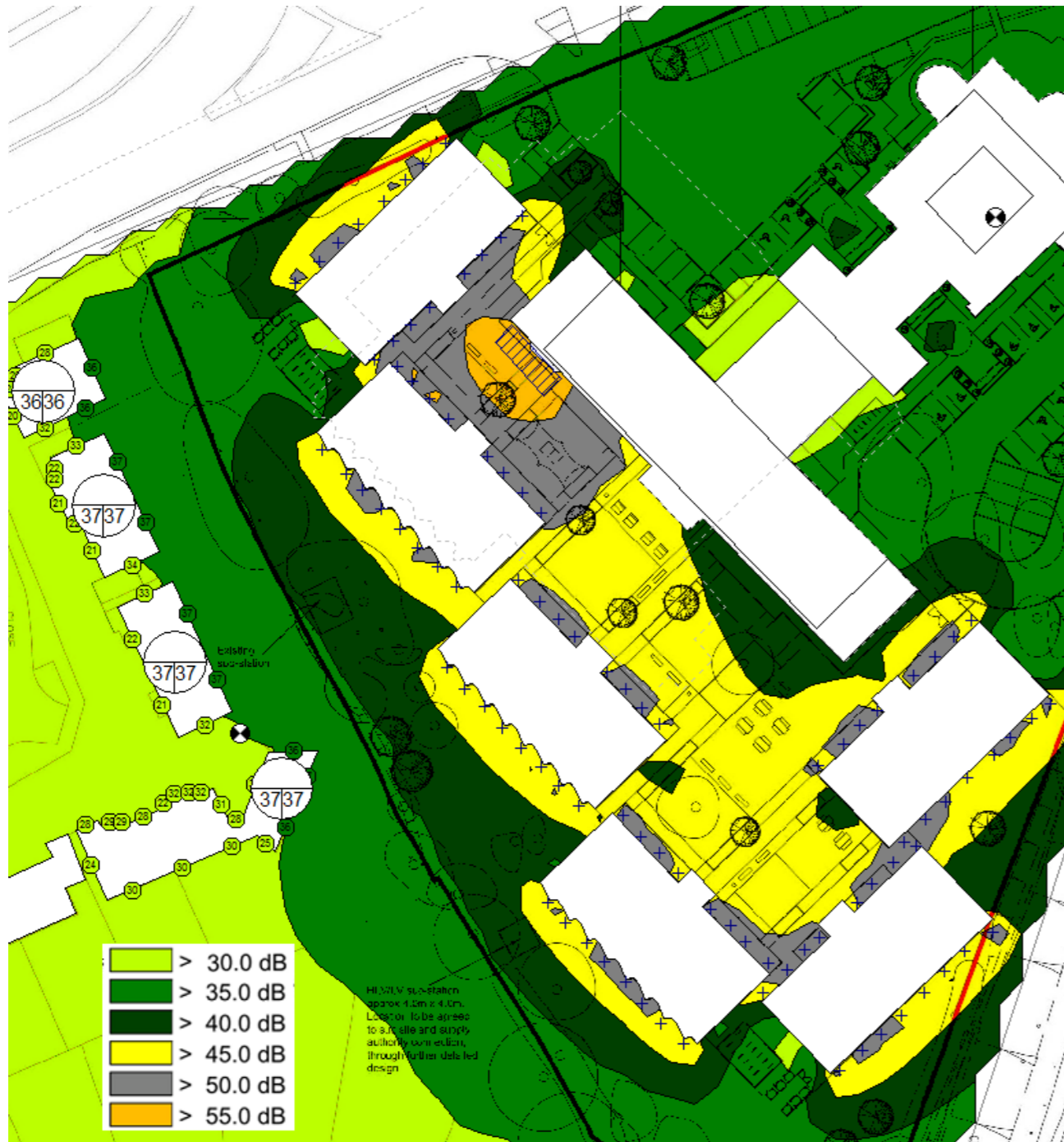
Figure 3: Sound contours at 4 m, showing the calculated specific sound level, L_{Aeq} , with all plant operating
