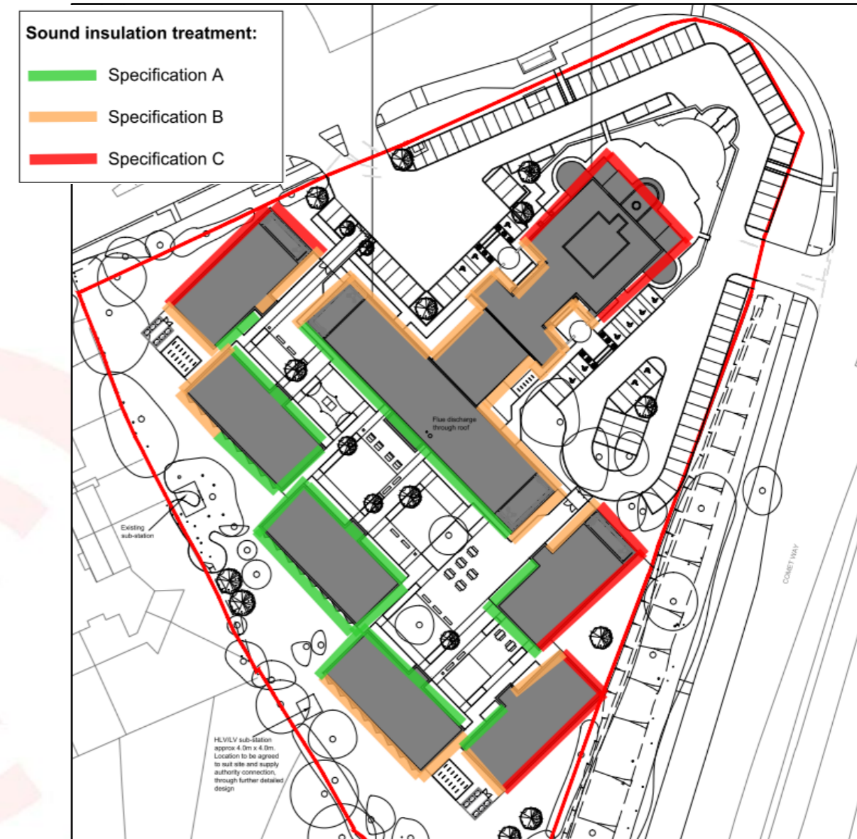
Figure 1: Site plan marked with sound insulation treatments
