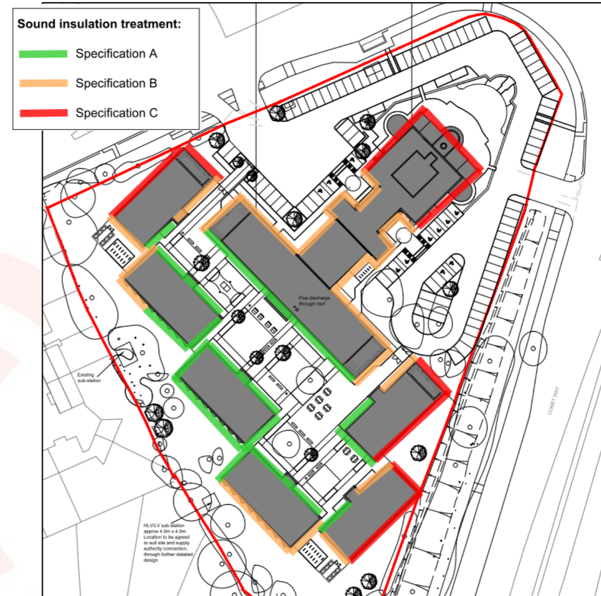
Figure 1: Site plan marked with sound insulation treatments
