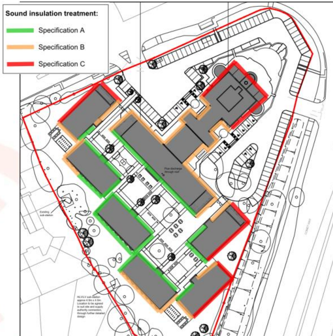
Figure 2: Plan highlighting specification requirements for each façade
