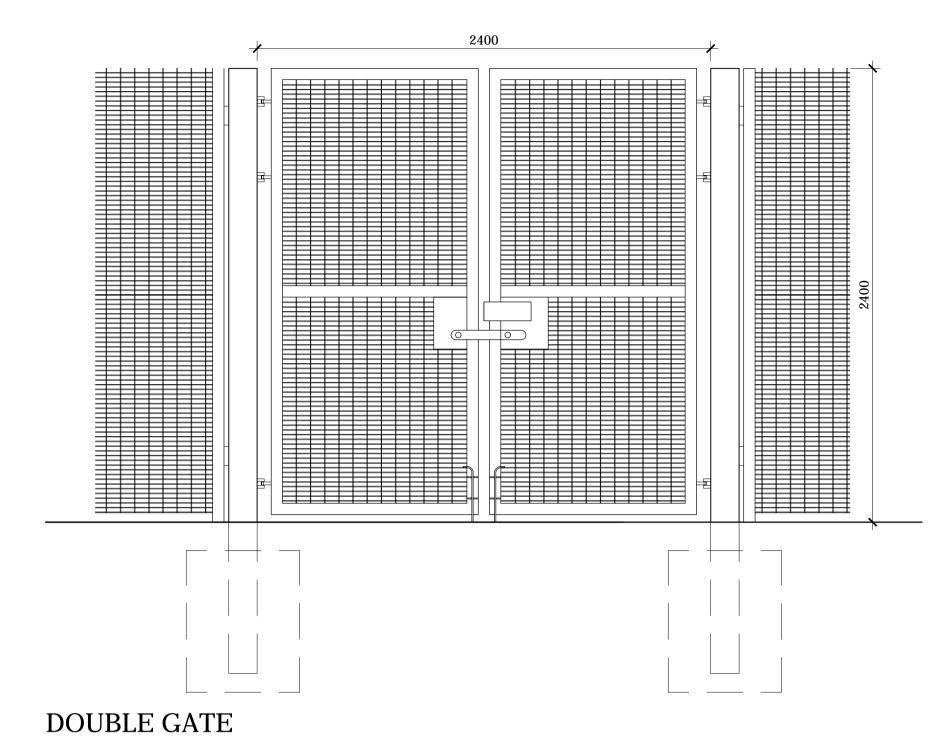
Double gate complete with europrofile cylinder lock with cover plate and drop bolt. 2.4m high paladin fence round perimeter of service yard as shown on site plan. Colour: PPC Green
