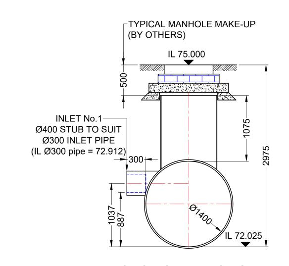
SECTION THROUGH Ø900 ACCESS SHAFT No.1 & INLET No.1 (WINCH ACCESS) SCALE 1:30
