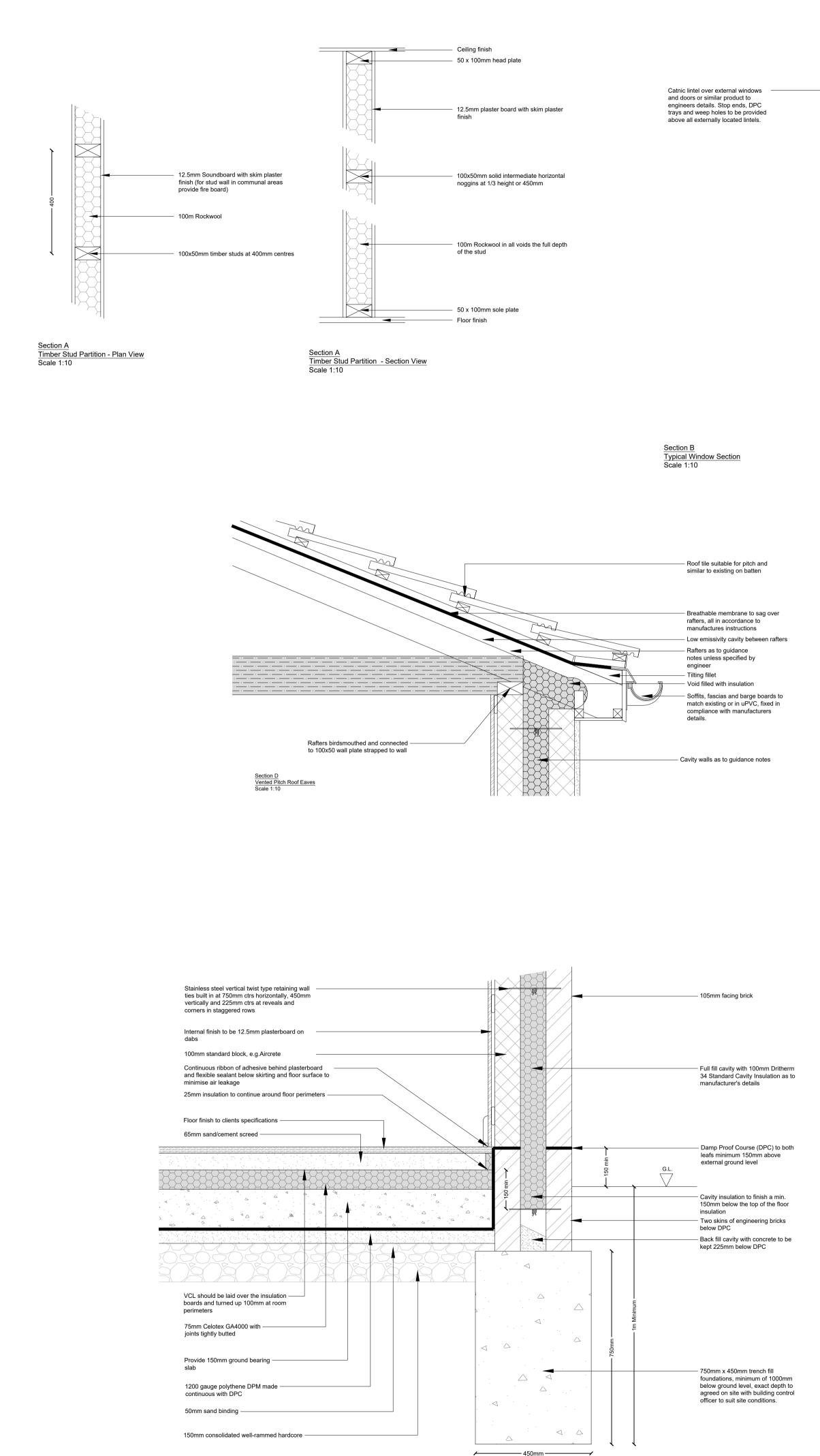
Section F Typical Concrete Slab / Foundation / External Wall Section Detail Scale 1:10
