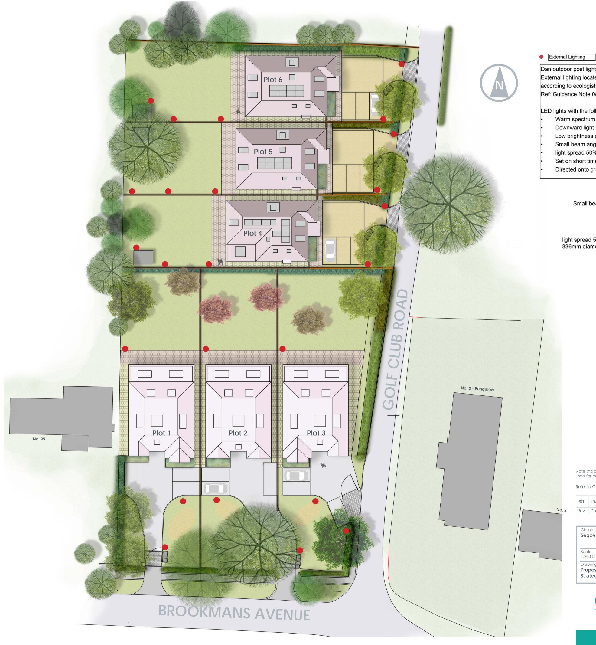
Dan outdoor post light (manufactured by Mark Slojd) External lighting located and selected to mitigate effects on bats, according to ecologists' recommendations.
