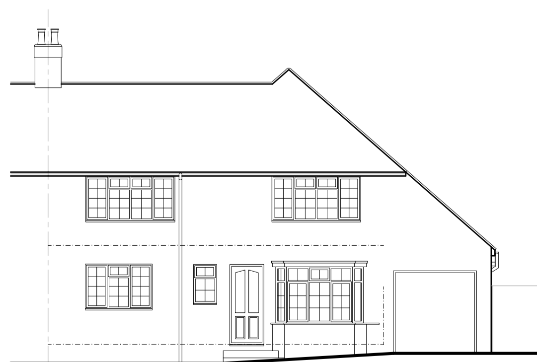
Front Elevation As Proposed 1:100
