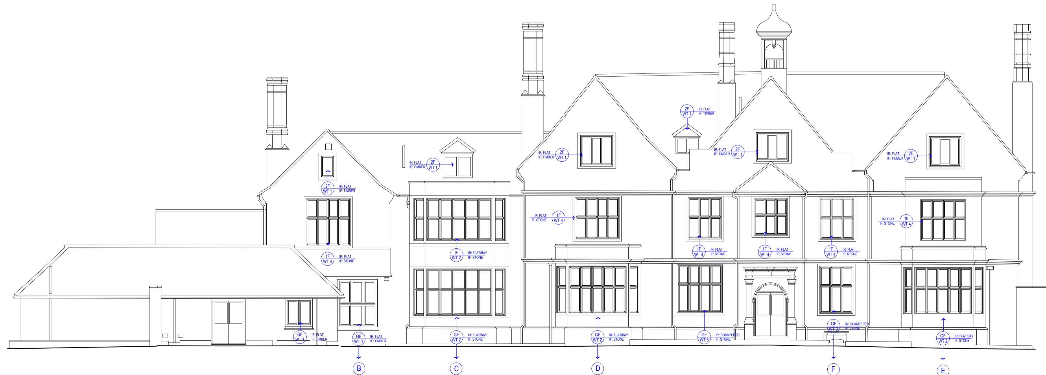
02] EXISTING FRONT / SOUTH ELEVATION @1:100
