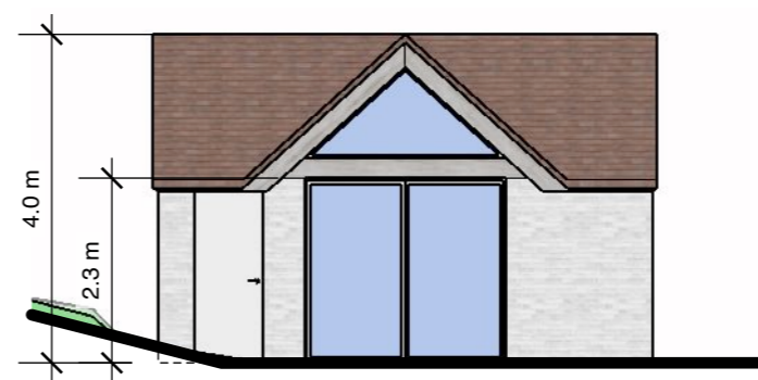
D Side (North) Elevation 1:100
