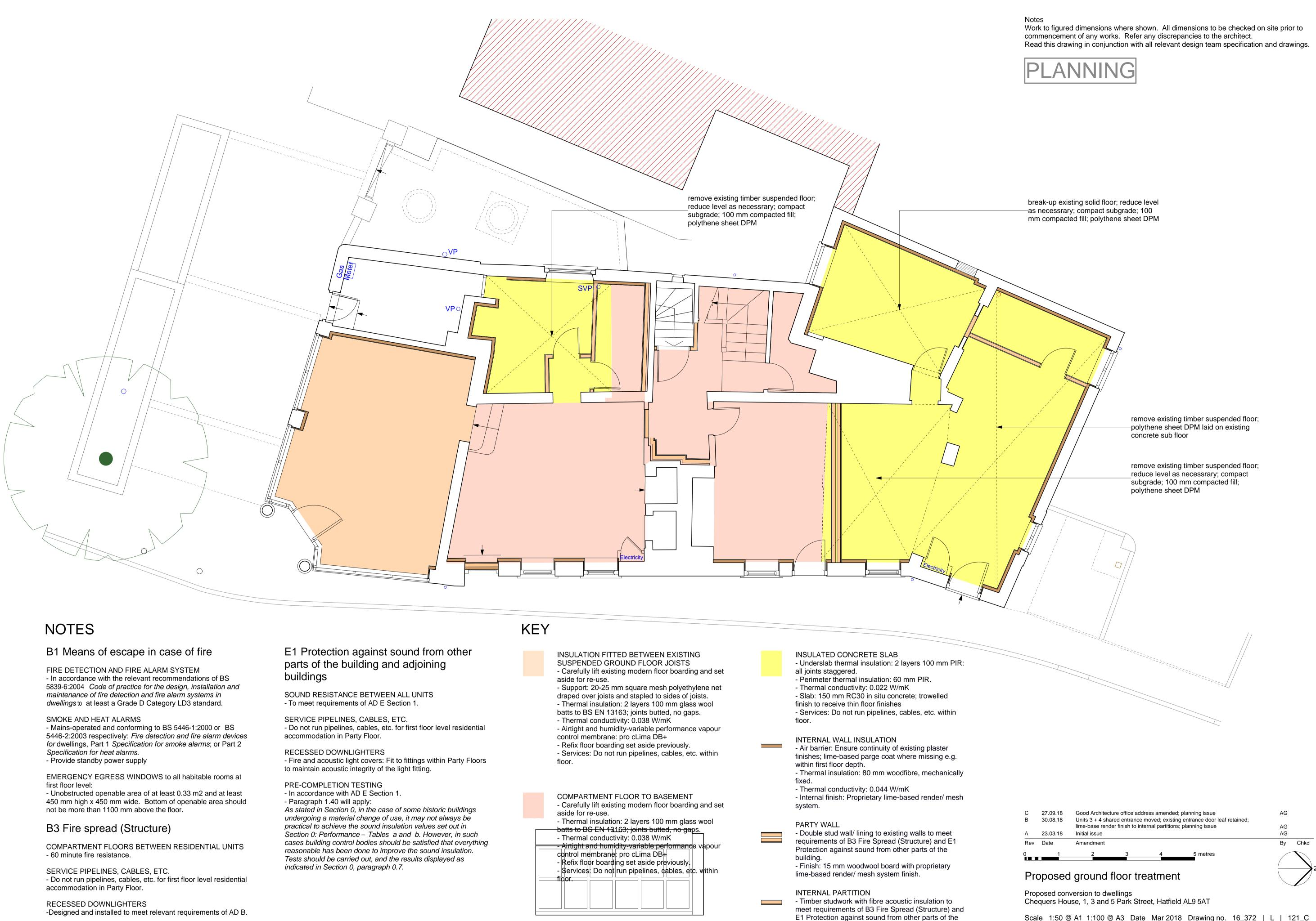
building. - Lining both sides: 15 mm woodwool board with proprietary lime-based render/ mesh system finish.
