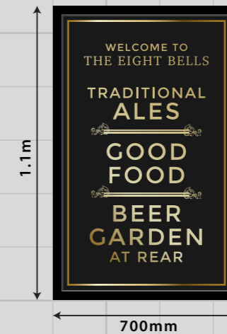
E TWO x new timber amenity boards with painted text. Size 700mm x 1.1m H.A.G 1m
