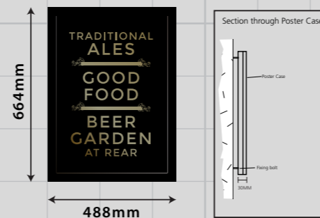
F ONE x new A2 poster case with painted text to back. Size. 488mm x 664mm H.A.G 1.1m.
