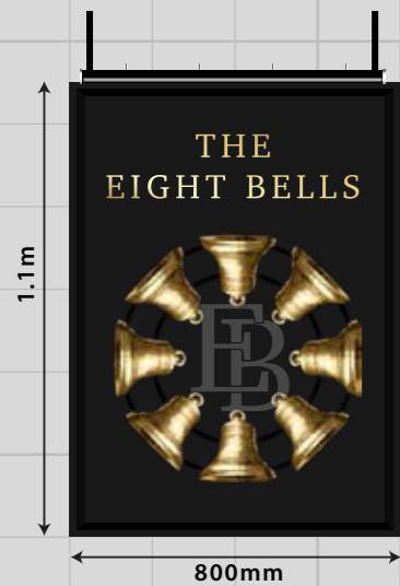
B ONE x new timber double sided projecting sign with painted detail, fixed to existing post sign, illuminated by new linolites. Size 800mm x 1.1m. H.A.G 3.4m.
