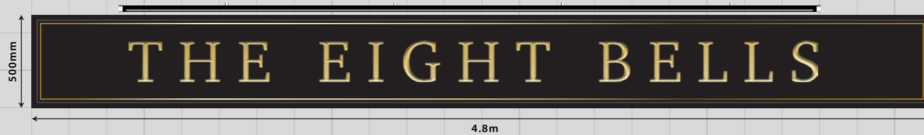
A ONE x new timber fascia with 10mm bevelled perspex letters, illuminated by trough light. Size 4.8m x 500mm. H.A.G 2.5m
