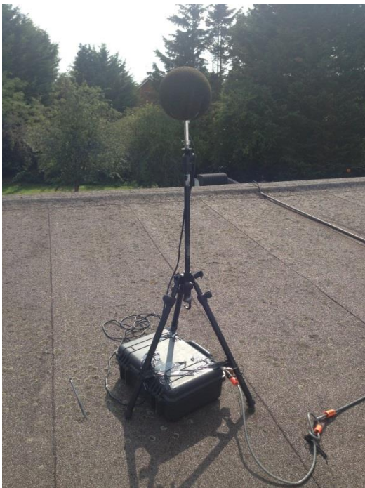
Figure 3 Photo showing microphone position at unattended measurement location 'B'
