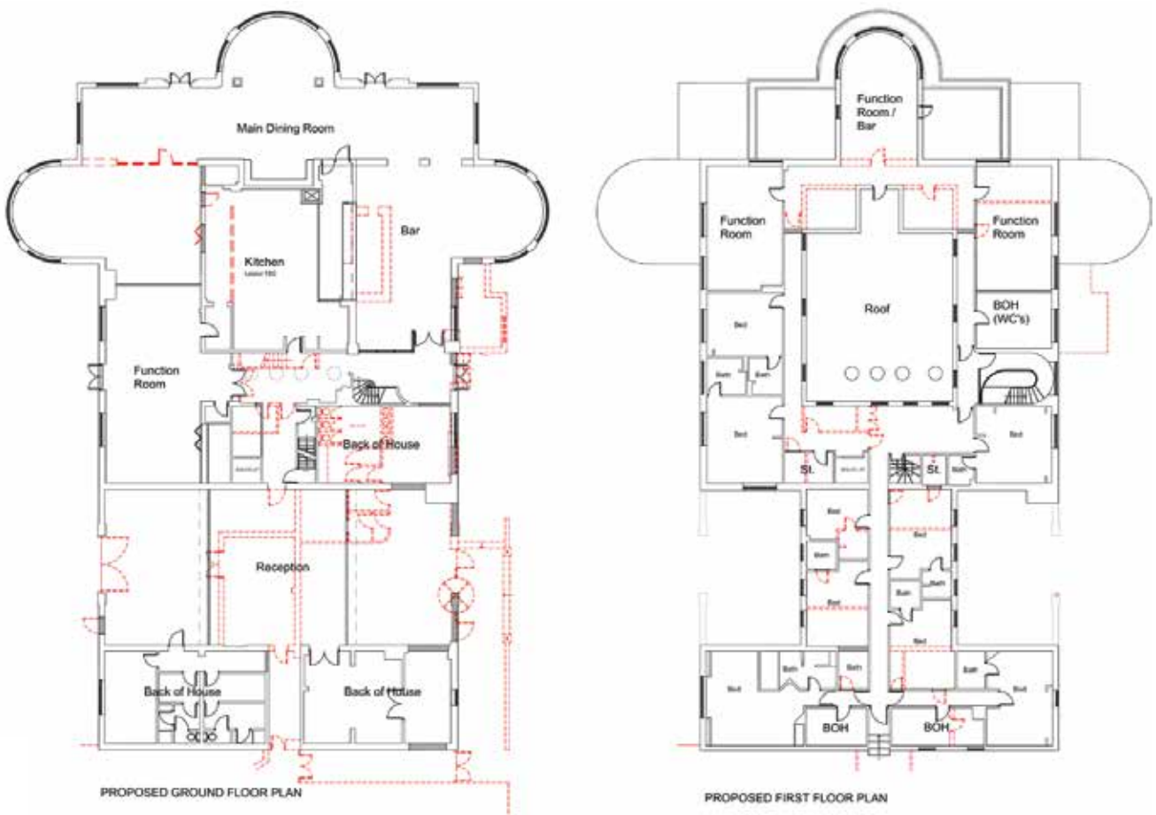
Proposed demolition plans
