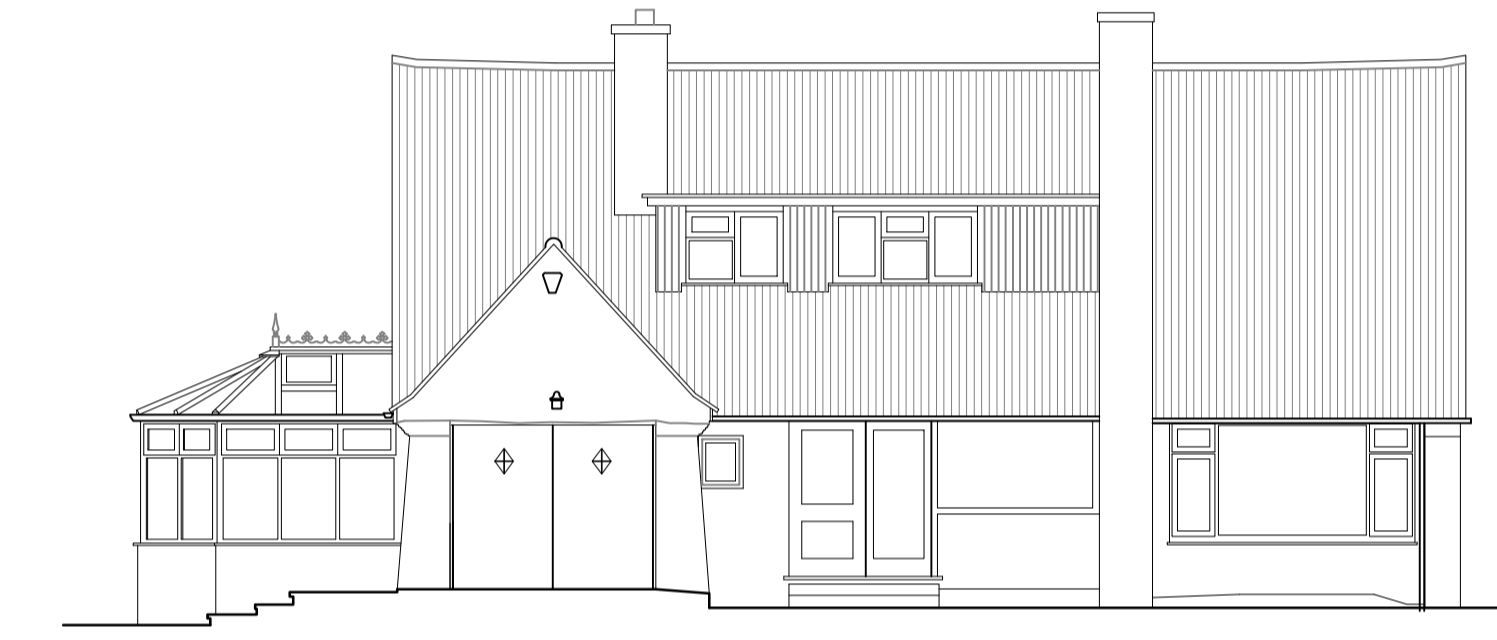
4 EXISTING FRONT ELEVATION 1:100
