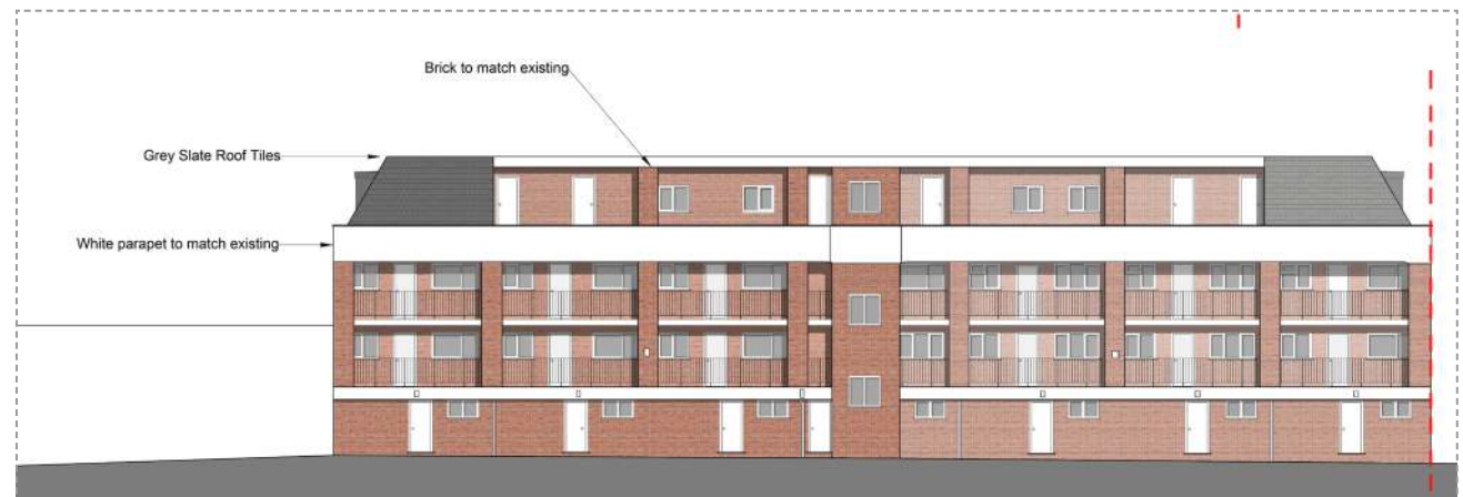
Proposed West Elevation
