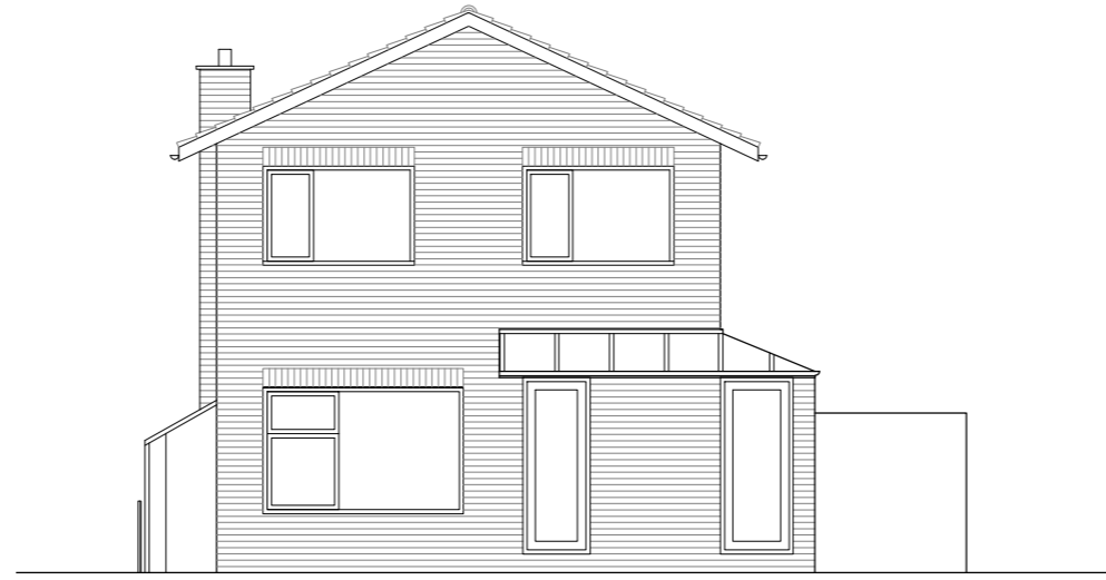
2 Existing Rear Elevation 1:100
