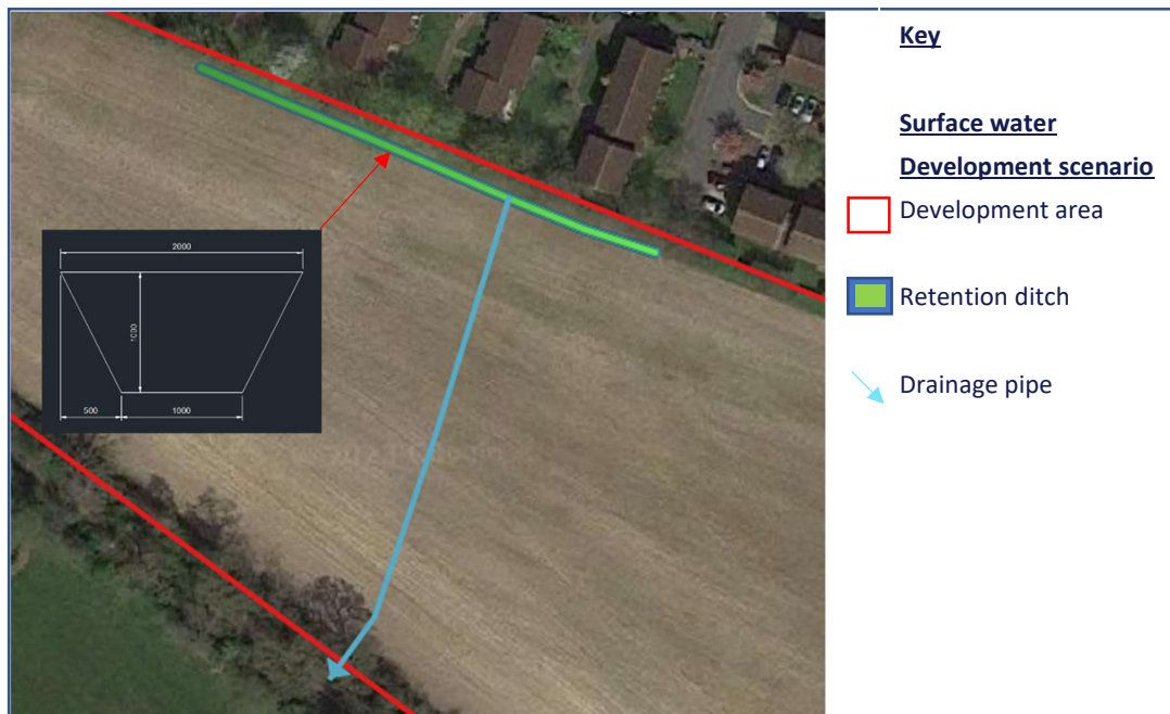
Figure 5-3 Proposed retention ditch and 450mm drainage pipe.
