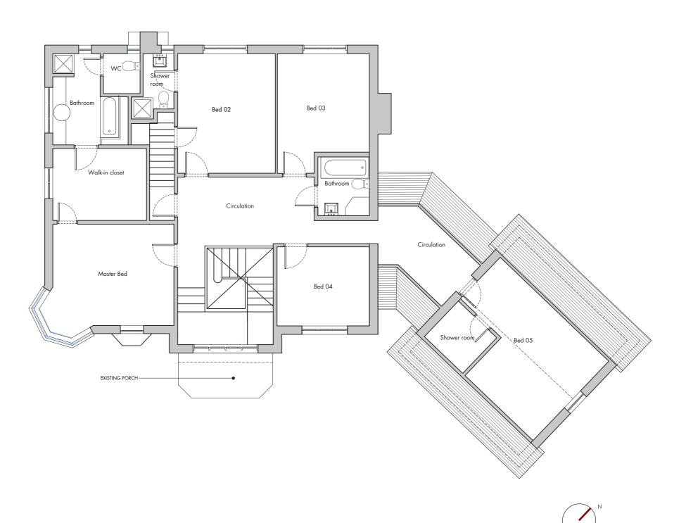
1\_Existing First Floor Plan
