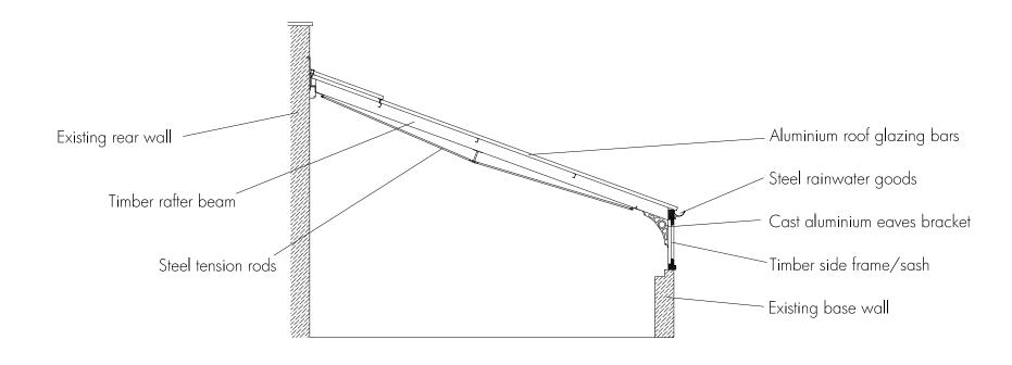
'Victorian' lean-to greenhouse Existing masonry base and rear walls with painted timber and aluminium glazed superstructure
