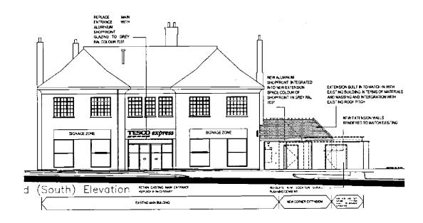
Figure 1 – Proposed South Elevation showing the Proposed Extension and New Shopfront
