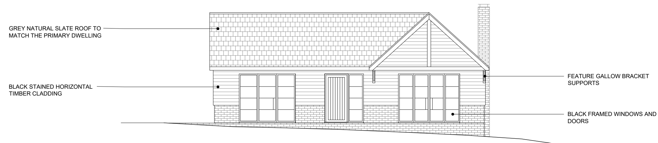
PROPOSED GRANNY ANNEXE - FRONT ELEVATION 1:100 @ A1
